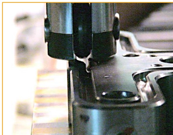
A wheel, mounted on the press ram, follows a groove cut in a metal plate. Sophisticated vision software generated the path for the robot to follow.
