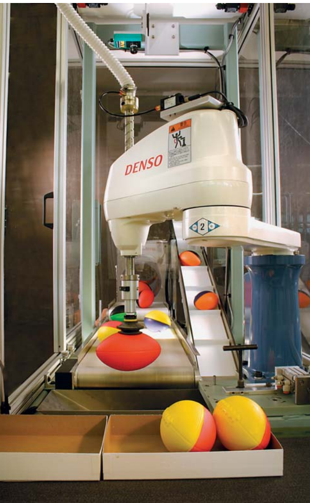
Vision guidance allows this robot to pick randomly oriented footballs from a moving conveyor belt and correctly place them in boxes.
