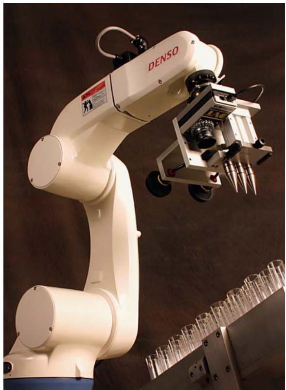
For robot guidance, cameras can be mounted to fixed positions in the cell, or they can be mounted directly to the robot.
