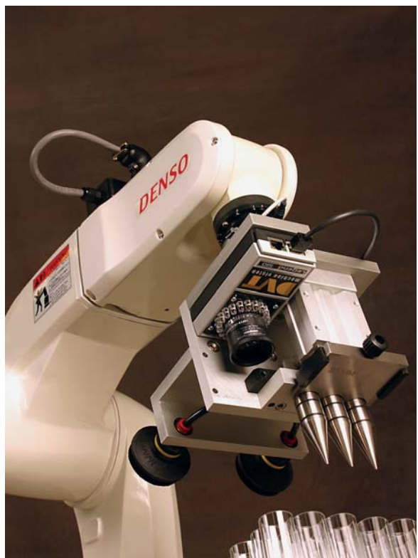
A vision-guided robot transfers glass tubes of varying diameters and heights to an assembly machine.
